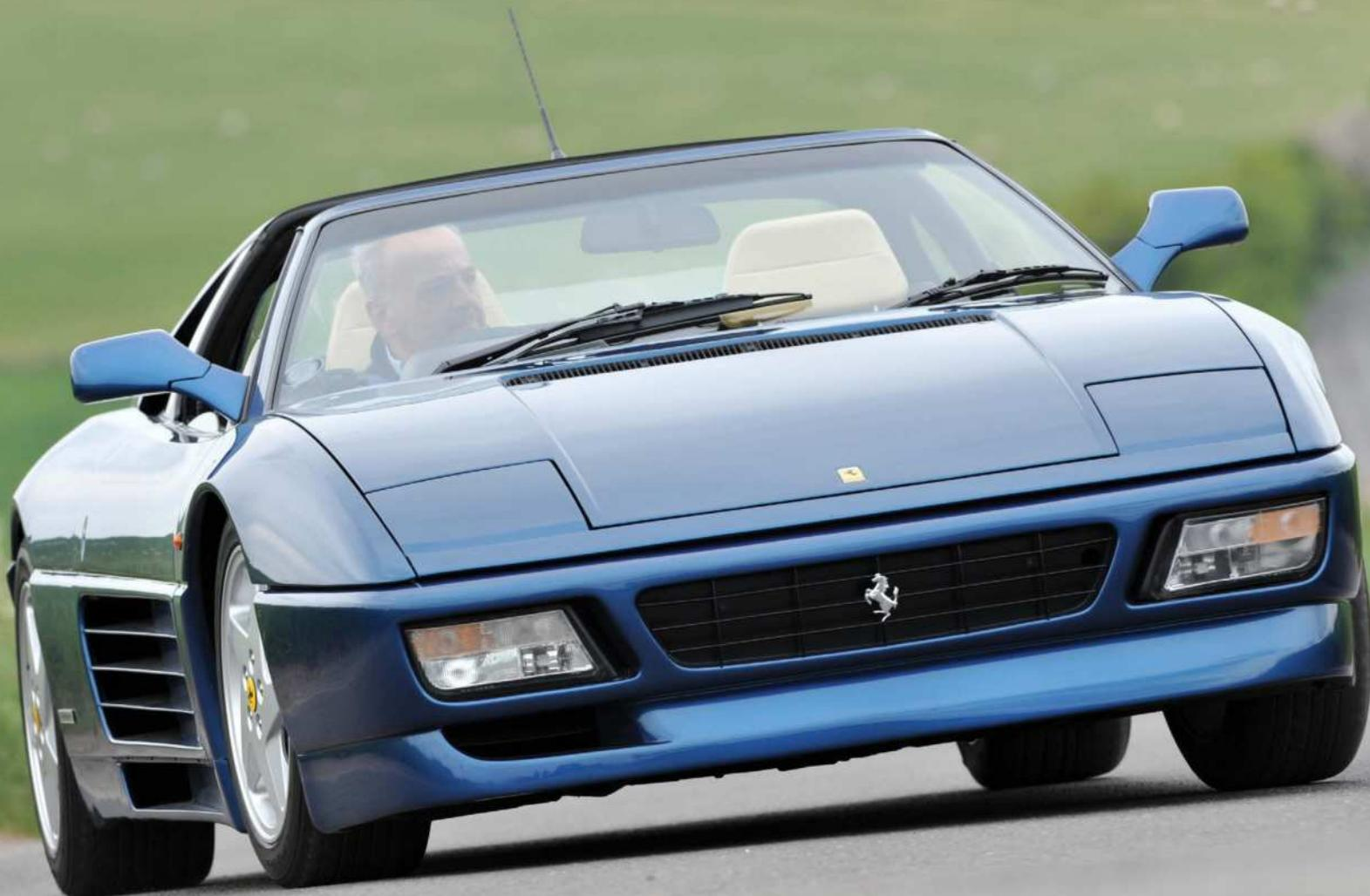
The 348 marked a new direction for Ferrari in that it abandoned spaceframe construction for a body formed of box sections, giving it 50 per cent greater torsional rigidity. The 348 tb was heavier than the old 328, tipping the scales at 1393kg (versus 1263kg). Yet its V8 engine had only 30hp more power and 15lb ft extra torque: the 348 had 300hp on launch (later upped to 320hp).
